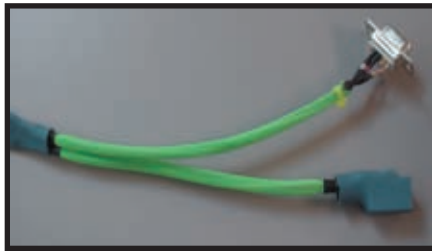
Photo 2 —We used an eight-pin header to make a programming cable that included an RJ-11 connector for in-circuit programming and a DE9 connector for access to the USART on the PIC18F4580.
