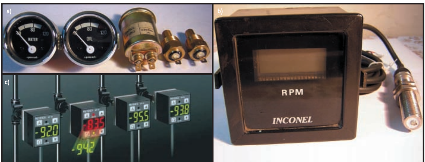
Photo 1 —I'm interested in several gauges and sensors: analog gauges with pressure and temperature senders (a), an RPM gauge with a magnetic pick-up sensor (b), and multipurpose digital pressure gauges with 5-V analog output (c).
